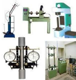
**UTM / TTM / CTM / HARDNESS / IMPACT / EXTENSOMETER**
